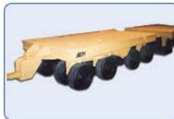
Automotive Die Handling Trailer 60 Ton Capacity
