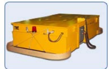
Battery Powered Die Handling Transfer Car
